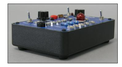
The Electrical/PWM/Fault Trainer is designed to introduce the concepts of Electrical Fundamentals, Pulse Width Modulation (PWM) Actuator Control, and Fault Diagnosis. The trainer is compact, self-contained, and provides a PWM output to view the signal on an oscilloscope.
