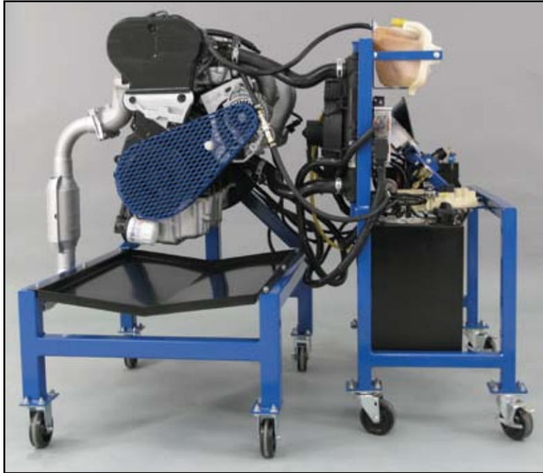
Engine Repair Trainer (model 90) connected to Engine Start Cart (model 91)
