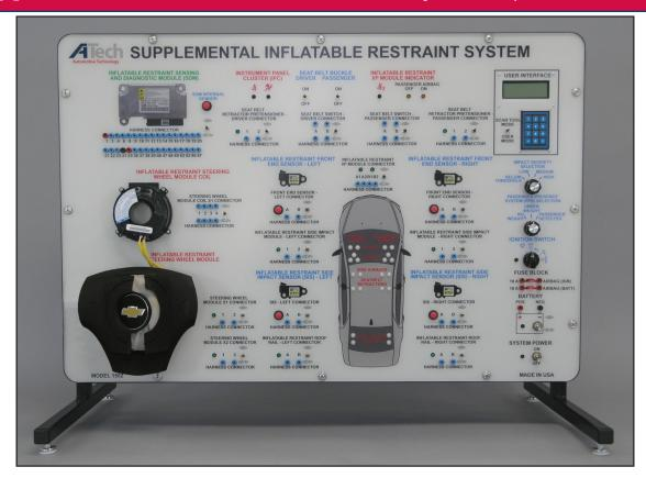
The trainer uses an actual SIR System that electrically responds and operates as in the automobile. The Air Bag portion of the trainer is a non-functional disarmed unit. The Supplemental Inflatable Restraint System is based on a CAN platform vehicle.
