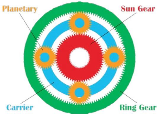
Figure 2: Planetary Gears
