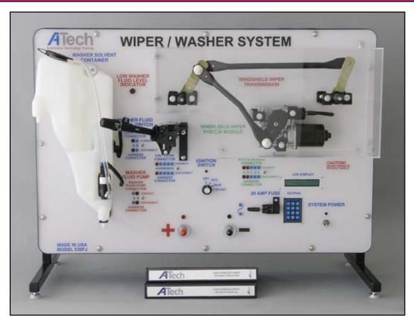
The ATech Wiper/Washer System Trainer (model 830Fj) is designed to teach computer and network controlled automotive witper/washer system operation. This trainer allows for instuctor demonstration, student hands-on reinforcement and troubleshooting practice. Powered by a 12VDC automotive battery or a 12VDC/23A power supply (not included).
